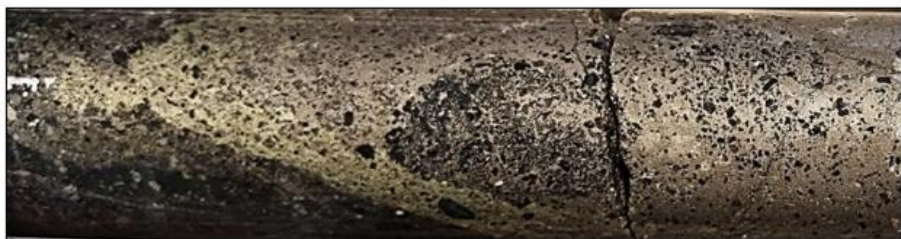
Figure 3: Massive pyrrhotite-pentlandite-chalcopyrite lens with sharp, cross-cutting contact to host peridotite unit. Note the fractionated chalcopyrite rich zone at the contact with host peridotite. From a 0.6 m sample that returned 1.51% Ni, 0.37% Cu, 0.15% Co, 180.0 m, 23RAN002. NQ diameter drill core.
