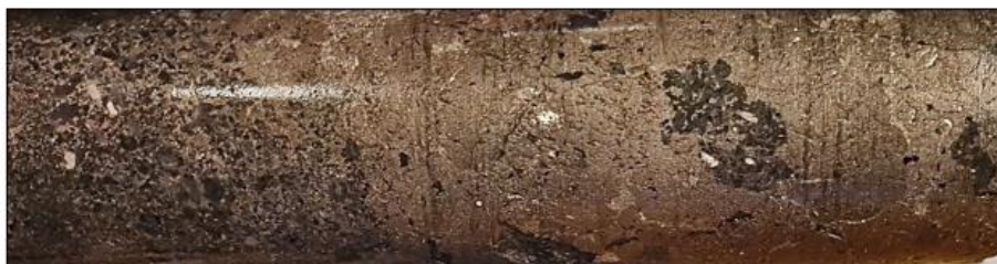
Figure 2: Massive and net-textured pyrrhotite-pentlandite-chalcopyrite with coarse pentlandite loop textures and rounded clasts of peridotite, from a 0.3 m sample that returned 1.71% Ni, 0.26% Cu, 0.15% Co, 176.54 m, 23RAN002. NQ diameter drill core.
