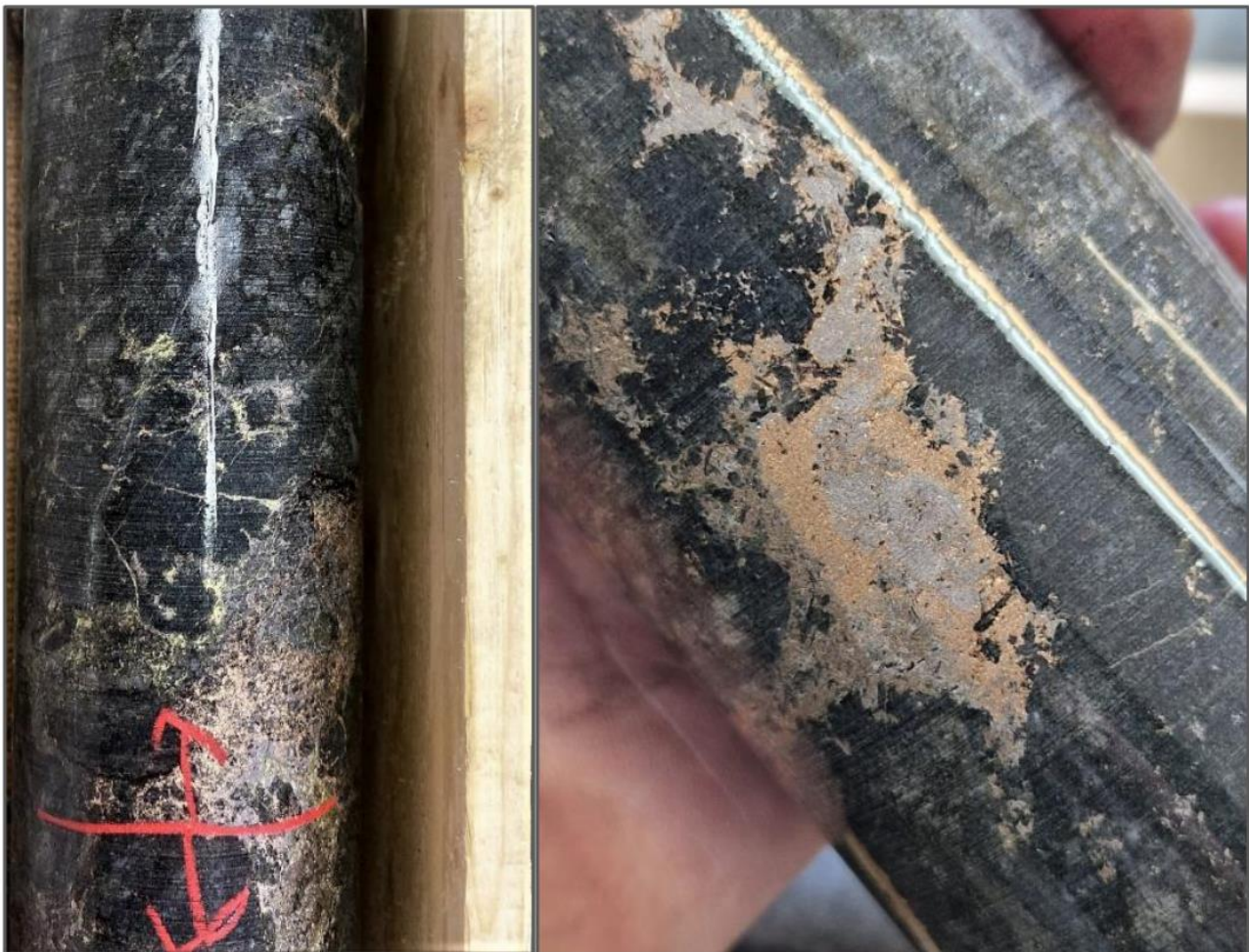
Drill hole LAI23001 showing nickel-copper sulfides (pyrrhotite, pentlandite and chalcopyrite) (Source: www.qxresources.com.au )
