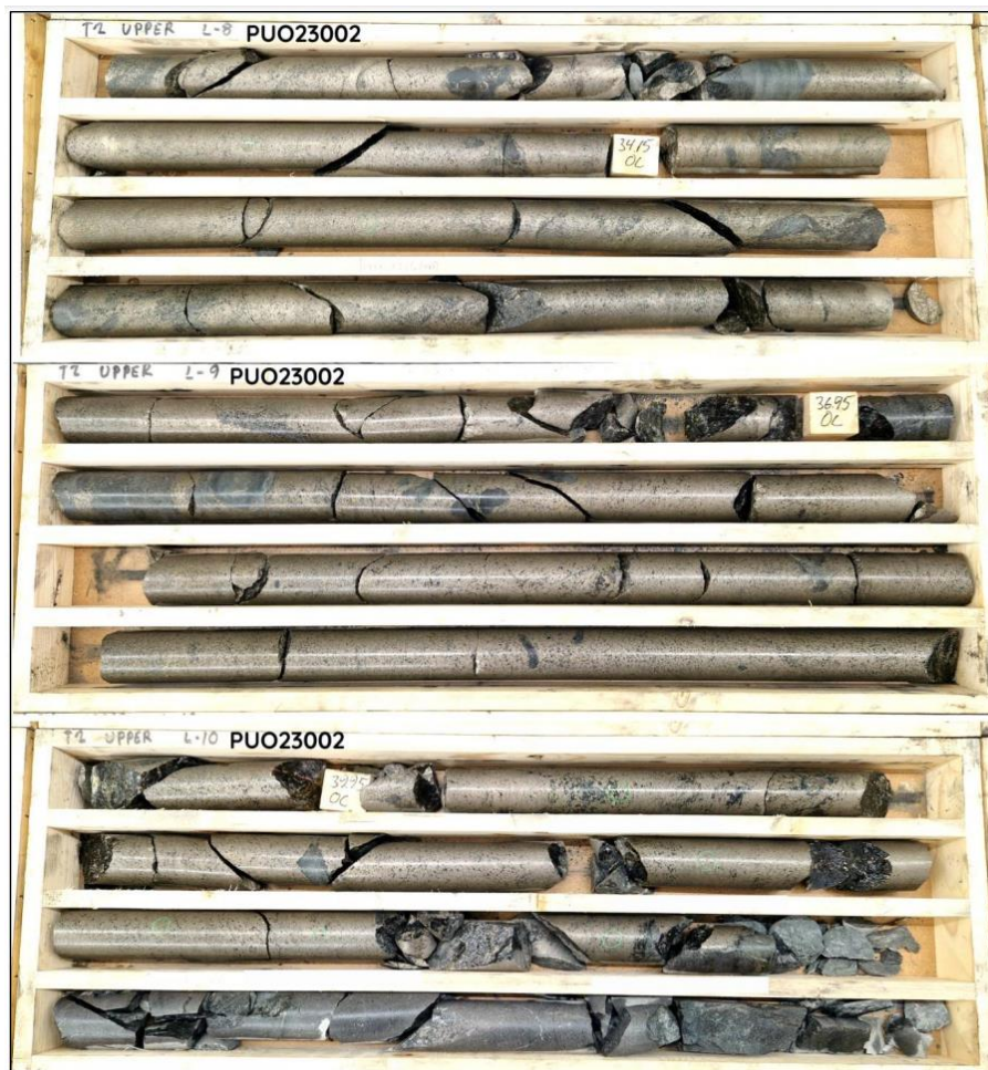
Massive sulfide in drill hole PUO23002 (Source: www.aviraresources.com.au )
